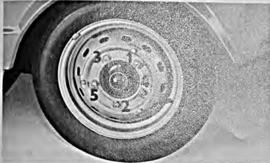
Tightening sequence for wheel bolts
